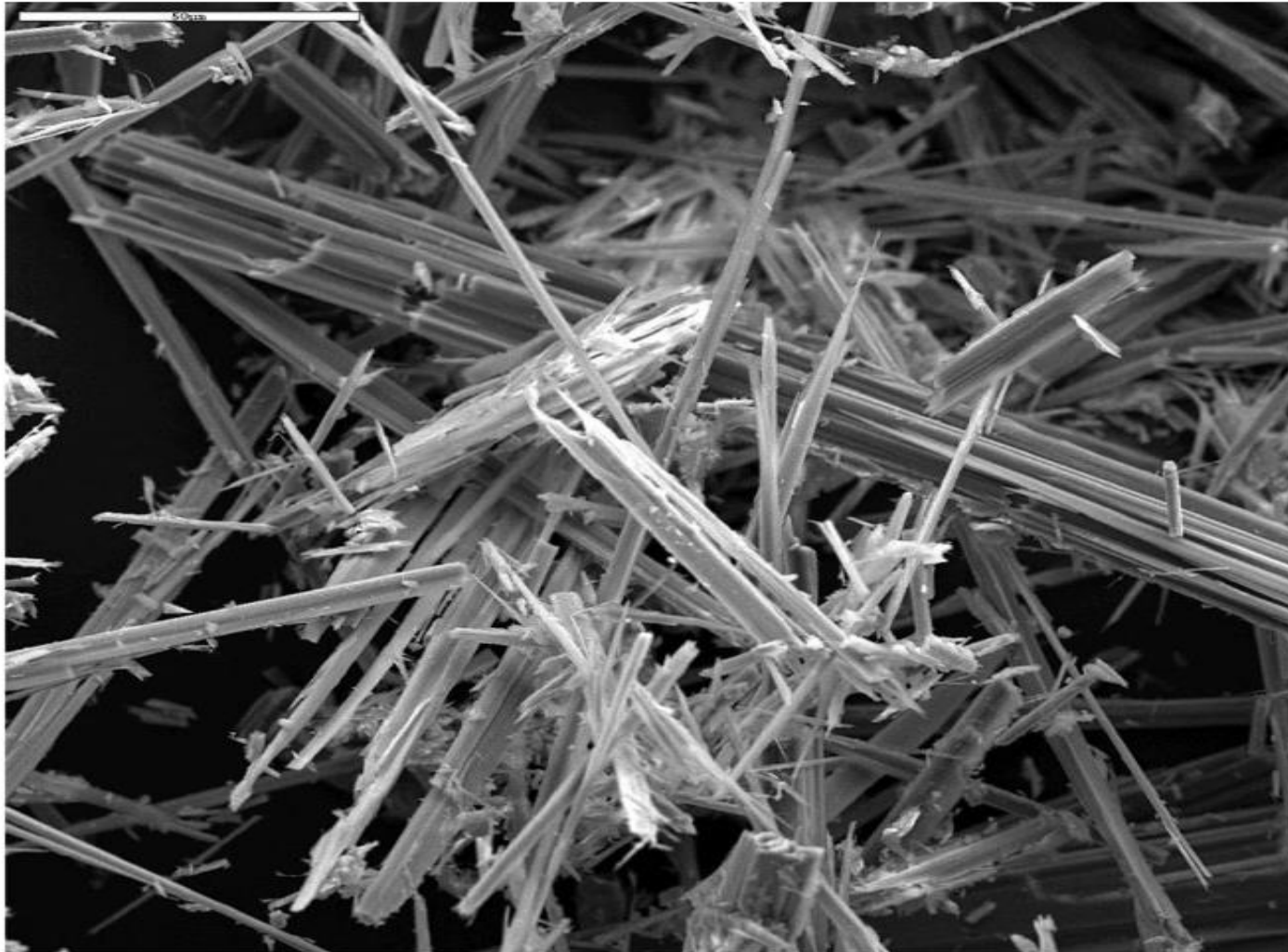
Asbestos fibers, image taken with a scanning electron microscope. Source: http://usgsprobe.cr.usgs.gov/picts2.html .
