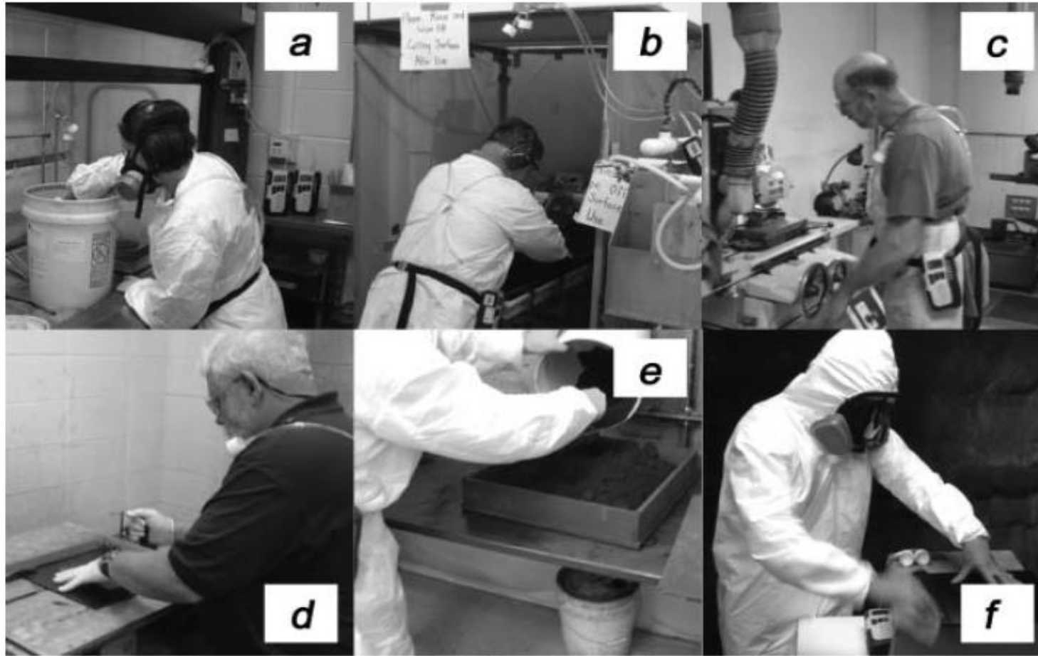
FIGURE 1. Photos of workers engaged in some tasks. (a) Weighing CNF's inside lab hood with sash in operating position; (b) Wet saw cutting composite inside canopy ventilated booth; (c) Surface grinding composite containing CNFs with LEV; (d) Table saw with wet diamond blade cutting composite (no controls); (e) Transferring CNF's to tray inside ventilated booth; (f) Hand sanding composite laminate material inside ventilated booth.
